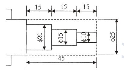
Working Materials: Mild steel, work size: 30 mm dia, Length: 50 mm dia, cutting speed = 600 r.p.m., feed = 150 mm/min, depth of cut should not exceed 2 mm.
