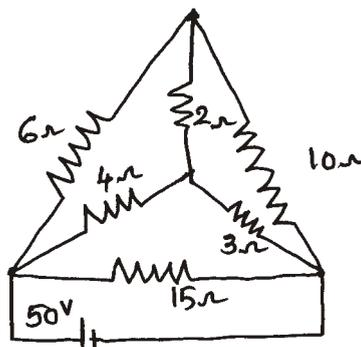
13. Determine the current in the 20 resistor in the circuit shown below, using superposition theorem :
